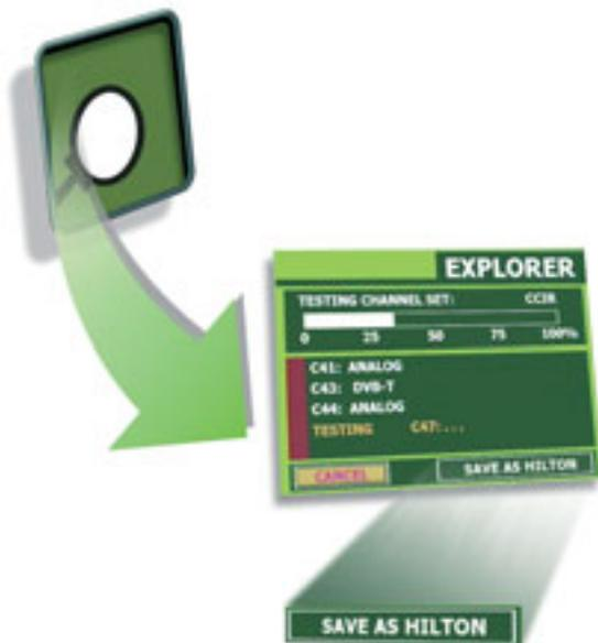
When the '**explorer**' key is pressed for a few seconds, a new spectrum exploration session begins. Unlike any other meter currently on the market, the **EXPLORER** makes a dynamic exploration of the spectrum, detecting all the channels in the swept band. This applies to the terrestrial and satellite television bands.
